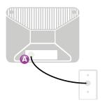
B Reconnect this end of the cable to the "Cable In" input on the back of the DTA.
